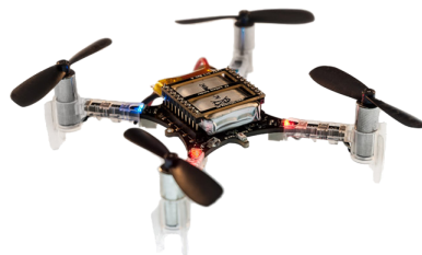
Fig. 1. The Crazyflie 2.0 nano-quadcopter.
